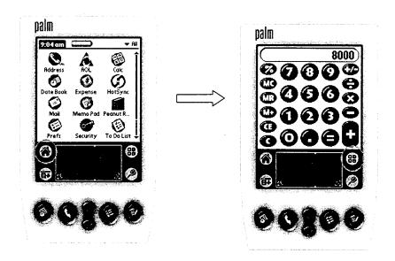
Both the Palm and Handspring devices have a liquid crystal display (LCD) screen which functions as both a display and a keyboard. It is described as the area which "[d]isplays the applications and information stored in the Visor [or Palm] handheld. It is touch sensitive and responds to a stylus." By touching the screen, a user can open applications, choose menu commands, select options in dialog boxes, and open the onscreen keyboard.
