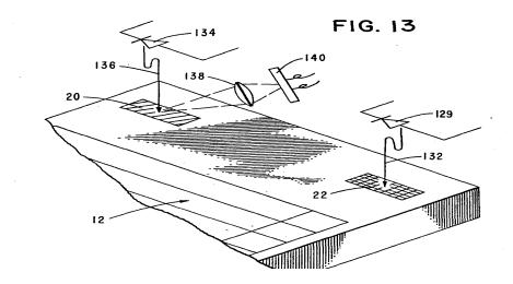
The patent explains that this configuration, in which both LEDs (labeled 129 and 134 in Figure 13) are on the I Module and data is transmitted by the P Terminal using reflection, allows the non-portable I Module to provide the power to the LEDs so that the smaller, battery-powered P Terminal is more energy-efficient.
