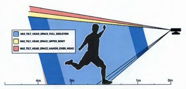
(D.I. 361 at 10; D.I. 366, ex. 21 at 10) The Xbox 360 and the Kinect together use an algorithm to track the user and determine the location of 20 points that correspond to various joints of the user's body, using a coordinate system centered at the Kinect sensor. (D.I. 333 at 6; D.I. 334, ex.
