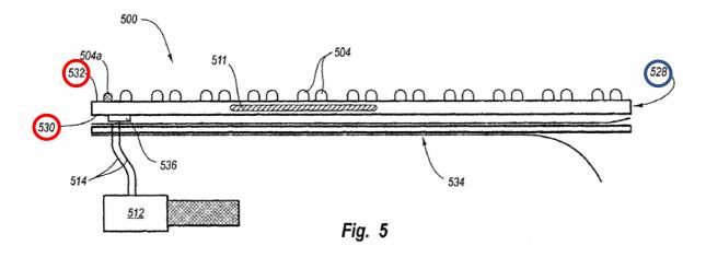
This figure is a side view of one embodiment, which would retrofit existing light fixtures. The specification identifies 530 as the attachment surface and 532 as the illumination surface (both circled in red above). ('747 patent at 9:19-20). These are opposite surfaces of the housing 528 (circled in blue above). Dr. Valencia Koomson, Plaintiff's expert, concludes that this figure depicts the attachment surface secured to the illumination surface via the side walls of the
