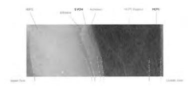
It is undisputed that the HDPE and HDPE Regrind layers are thermoplastic polymer layers and that the EVOH layer is a fuel-impermeable barrier layer. (See D.I. 236 at 27) It is further undisputed that at least some of the barrier layer and at least some of the HDPE Regrind layer enter the orifice. (See D.I. 224 at 24; D.I. 236 at 27) The central dispute is whether the "outer layer" is the HDPE Regrind layer, the HDPE layer, or both.
