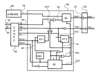
('730 patent, Fig. 4A.) "Block 34" of this figure, which corresponds to the "framer," is denoted by the dashed line. Other components of this figure that have been the subject of expert testimony are block 50, which is a "data selector"; block 62, a "clock generator"; and block 30 (not part of the framer), which is a "CODEC." An accompanying text in the patent's specification describes how
