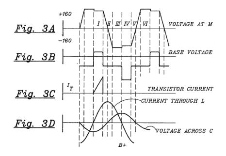
"As shown in FIG. 3c, current-flow in transistor 43 terminates at the end of period I." (*Id.*, 4:27–29). This figure shows a transistor current pulse having a duration "distinctly shorter" than half of the complete cycle of the alternating voltage, which is shown in Figure 3A (time periods I–VI).
