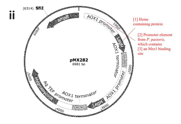
If Ginkgo and Motif's construction were correct, the corresponding embodiment would also contain a sequence encoding the Mxr1 protein linked to a separate promoter. An annotated version of Figure 2(ii) embodying the first part of claim 1 under Ginkgo and Motif's construction is shown below: <sup>9</sup>
